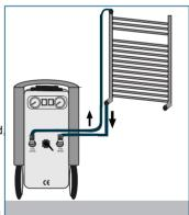
If the pump is not used for a long time, it will be blockaged. To avoid this, run the pump once a week.
